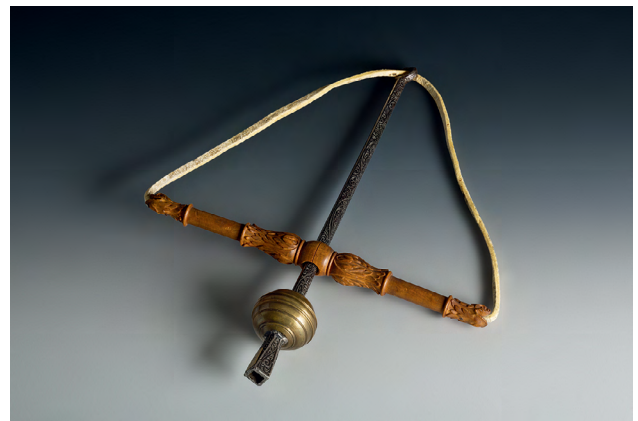
Figure 4 Pump drill ( Rennspindel ), Germany, c.1570, Iron, brass weight, wood, leather strap, L. 30.4 cm, W. 23 cm, Flywheel d. 3.9 cm, Rüstammer, inv. N° P 0224.
