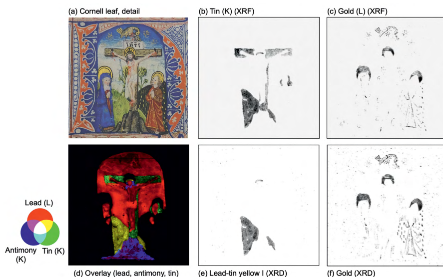
Figure 6 XRF and XRD maps for Cornell leaf. (a) Detail of the scanned area. (b) Tin (K) XRF. (c) Gold (L) XRF. (d) Overlay of lead (L) in red, tin (K) in green, and antimony (K) in blue, with color key to the left. (e) Lead-tin yellow type I XRD. (f) Gold XRD.
